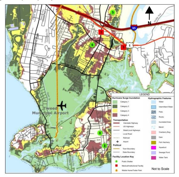
Figure 3: Hurricane Surge Inundation Mapping (Source: CT Division of Emergency Management)
